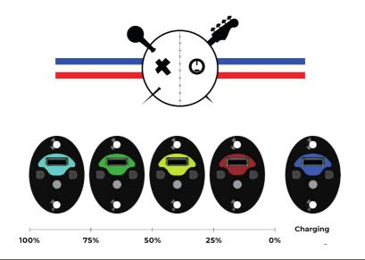
**START:** Connect the jack, a click on the button will turn on the B.M.S and show the amount of battery remaining.
